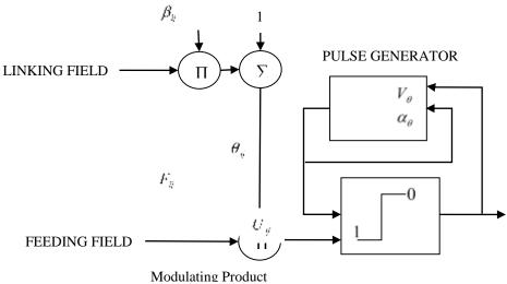
Fig. 3 Simplified model of PCNN neuron
