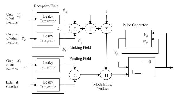
Fig. 2 Basic model of PCNN neuron
